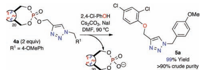
Scheme 2. Triazolization of 2,4-Cl-PhOH Utilizing OTP 4a
